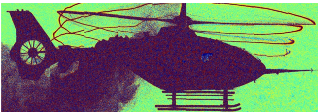
Fig. 2 BOS image of an EC 135 in forward flight, measured by Wolf et al. (2022)
