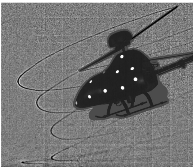
Fig. 17 Vortex system around a model helicopter during takeoff, for setup parameters see Bauknecht et al. (2019)
