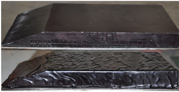
Fig. 2 Fuel slab configuration used in this research, before (top) and after (bottom) combustion test
