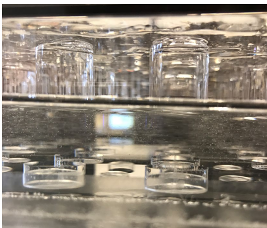
Fig. 2 Experimental cell partly filled with working fluid, note the tiny air bubbles entrained in the flow
