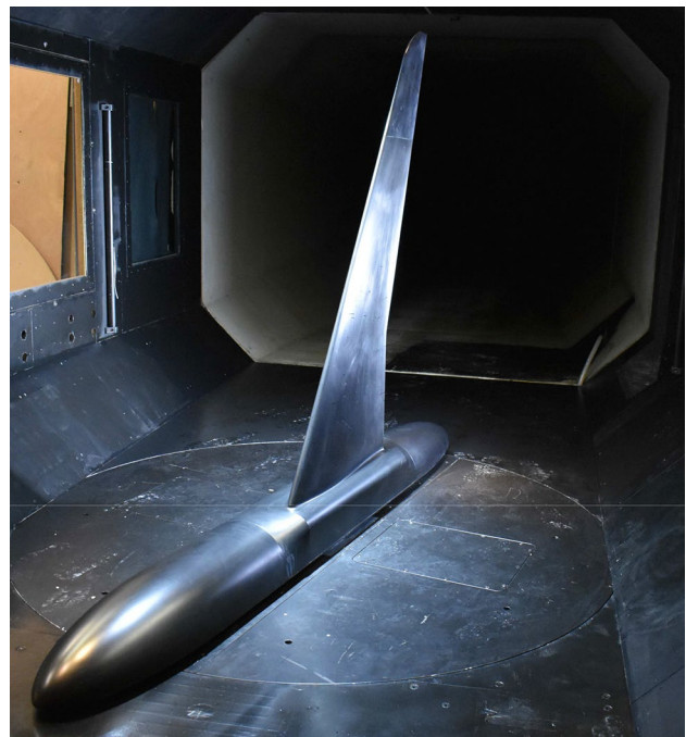
Fig. 1 Semi-span model installed in dH working section
