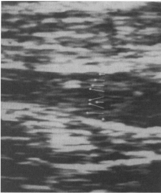
Fig. 13 An early example of blood flow measurement using correlation of B-mode images. The image shows a human popliteal vein, acquired using a 10 MHz scanner. The transducer position is located at the top of the image. The vectors represent the result of the local correlation search. Reproduced from Trahey et al. (1987). ©1987 IEEE. Reprinted, with permission, from IEEE Transactions on Bio-medical Engineering
