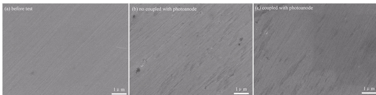
Fig.27 SEM images of 304SS blank (a); no protection (b); and coupled with Fe-doped TiO 2 (c)
