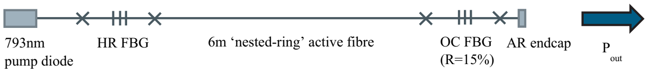
Fig. 3 A typical fibre laser cavity using the nested-ring fibre
