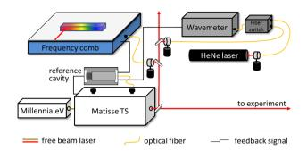
**Fig. 1** Laser system used for the investigations. Pumped by a Millennia eV Nd:YAG laser, light between 700 and 1000 nm can be generated with a Matisse Ti:Sa laser. A small fraction of the fundamental light is fed into the wavelength meters and the frequency comb. The laser frequency determined with these devices can be used for the long-term stabilization of the Matisse's reference cavity
