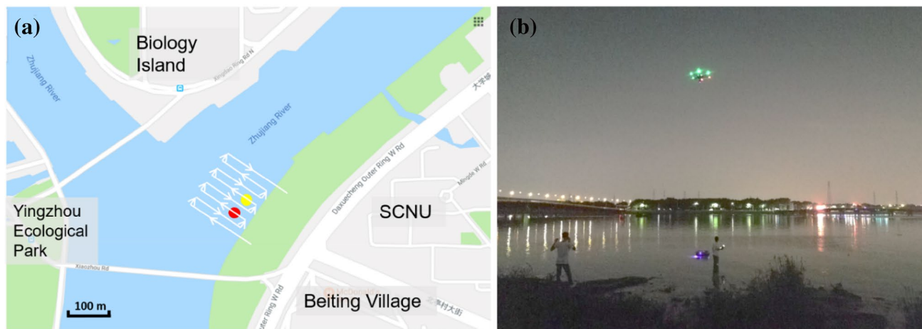
Fig. 5 a Map of the drone-based fluorosensor scanning over the Zhujiang river; b photo of the in situ measurements with the drone flying over the river and the exciting laser beam hitting the surface and inducing fluorescence
