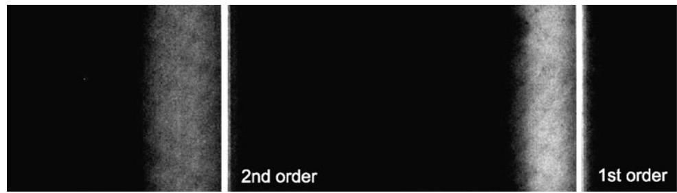
Fig. 9 Spectrum of a Ni-like samarium X-ray laser obtained with a flat-field spectrometer. The lasing line at 7.36 nm is visible in the first and second order of the spectrum
