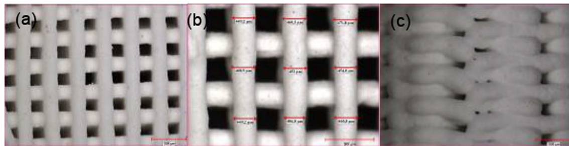
Fig. 3 Optical microscope images of the bare 13–93 bioactive glass scaffolds fabricated in the study; a , b top view, c side view
