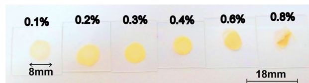
Fig.11 Visual effect of increased GTA concentration on CSNC thin films (standard cover slips have a dimension of ~ 18 × 18 mm and the thin films were found to have diameter of ~ 8 mm)
