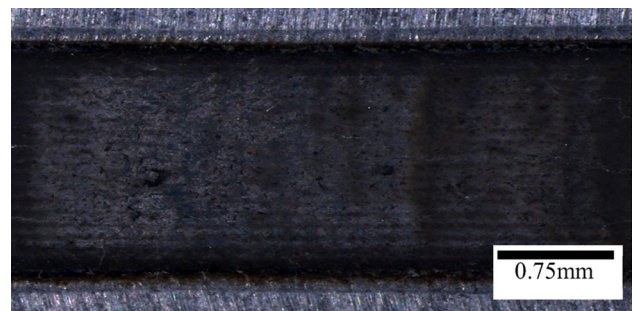
Fig. 6 Surface of the laser run face after treatment with WC powder using 1.5 kW laser power, scan rate 0.5 m/s, AlSi 7 Cu 2 cast alloy
