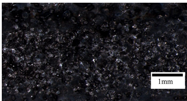
Fig. 4 Surface of the laser run face after treatment with WC powder using 1.5 kW laser power, scan rate 0.25 m/s, AlSi 7 Cu 2 cast alloy
