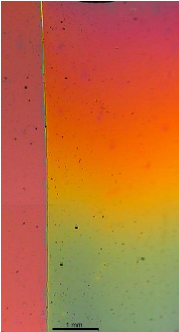
Fig. 4 Photograph of a SiO 2 -Si sample after surfactant sputtering using Xe ions and Al surfactants. Ion-irradiation was done using 5 keV Xe with 3 \times 10^{16}/\text{cm}^2 incident at \alpha = 80^\circ from below. The Al sputtering target was positioned above the upper boundary of the sample inclined at \beta = 30^\circ to the ion beam direction. The left part of the sample was not exposed to the ion beam and has an oxide thickness of 450 nm. The right part was exposed to the ion beam and simultaneously covered with Al surfactants during erosion with area density increasing from the bottom to the top. The interference colors from blue-green (bottom) over yellow to magenta indicate the increasing residual thickness of the SiO 2 layer from 310 to 430 nm
