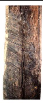
Fig. 12 An example of toolmarks from a saw on a bridge element (photo Archeologisch Centrum Leiden/BIAX *Consult*)
