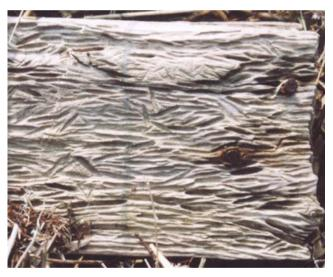
**Fig. 13** Infestation with aquatic invertebrate on non-archaeological material, identical to the traces found on the elements of the bridges (photo BIAX *Consult*)
