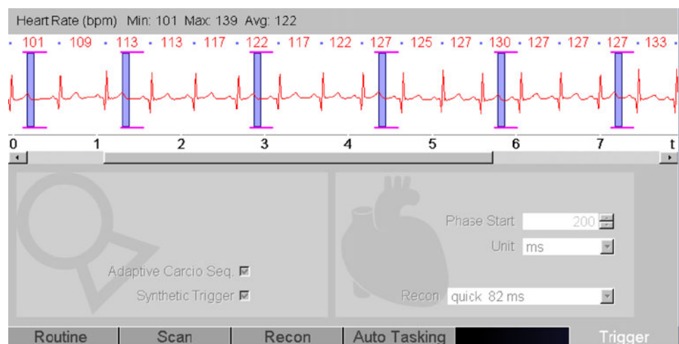
Fig. 8 An ECG-trace with an acquisition triggered on every third cardiac cycle
