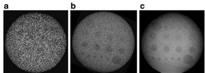
**Fig. 4a–c** The detectability of low-contrast details depends on reconstruction parameters and dose. **a**, **b** High- and low-resolution reconstructions are associated with high and low noise, respectively. **c** An increase of dose, compared with **a**, **b**, leads to lower noise and results in improved low-contrast detectability (see text)
