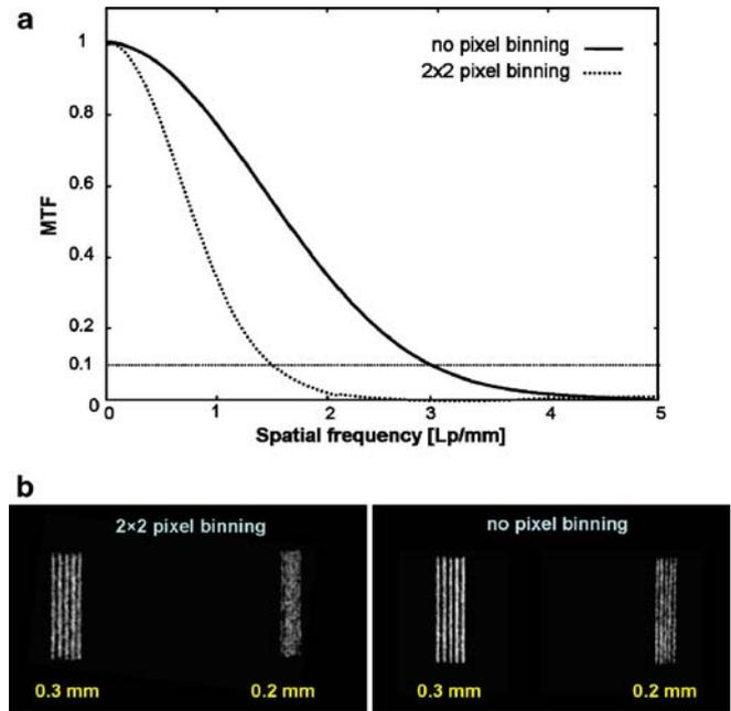
**Fig. 3** Superior spatial resolution is demonstrated **a** by MTF and **b** by bar pattern measurements. Pixel binning (see text) has a strong effect, but resolution generally exceeds that of clinical CT
