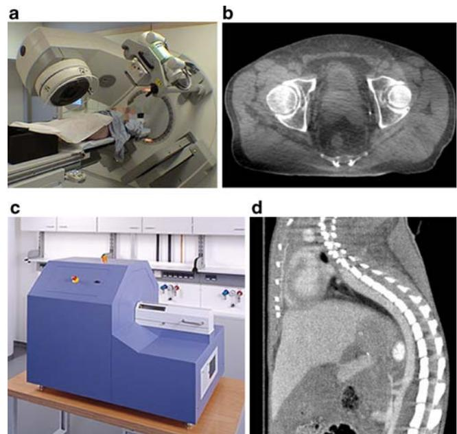
**Fig. 7a–d** Dedicated FD-CT scanners. **a, b** X-ray source and FD attached to a rotating linear accelerator for CT imaging of radiotherapy patients on the treatment couch. (Courtesy of D. Jaffray, Toronto.) **c** Micro-CT scanner for fast low-dose in-vivo imaging of small animals. **d** A 90-s scan of a mouse at 80- $\mu$ m resolution and 130 mGy after contrast medium injection
