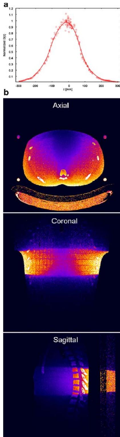
**Fig. 5a, b** Dose in FD-CT. **a** Dose profile along the central axis of a 600-mm long PMMA phantom of 32-cm diameter for 200-mm z-collimation. **b** Dedicated Monte Carlo tools provide exact 3D dose distributions for any CT scan and scan parameters
