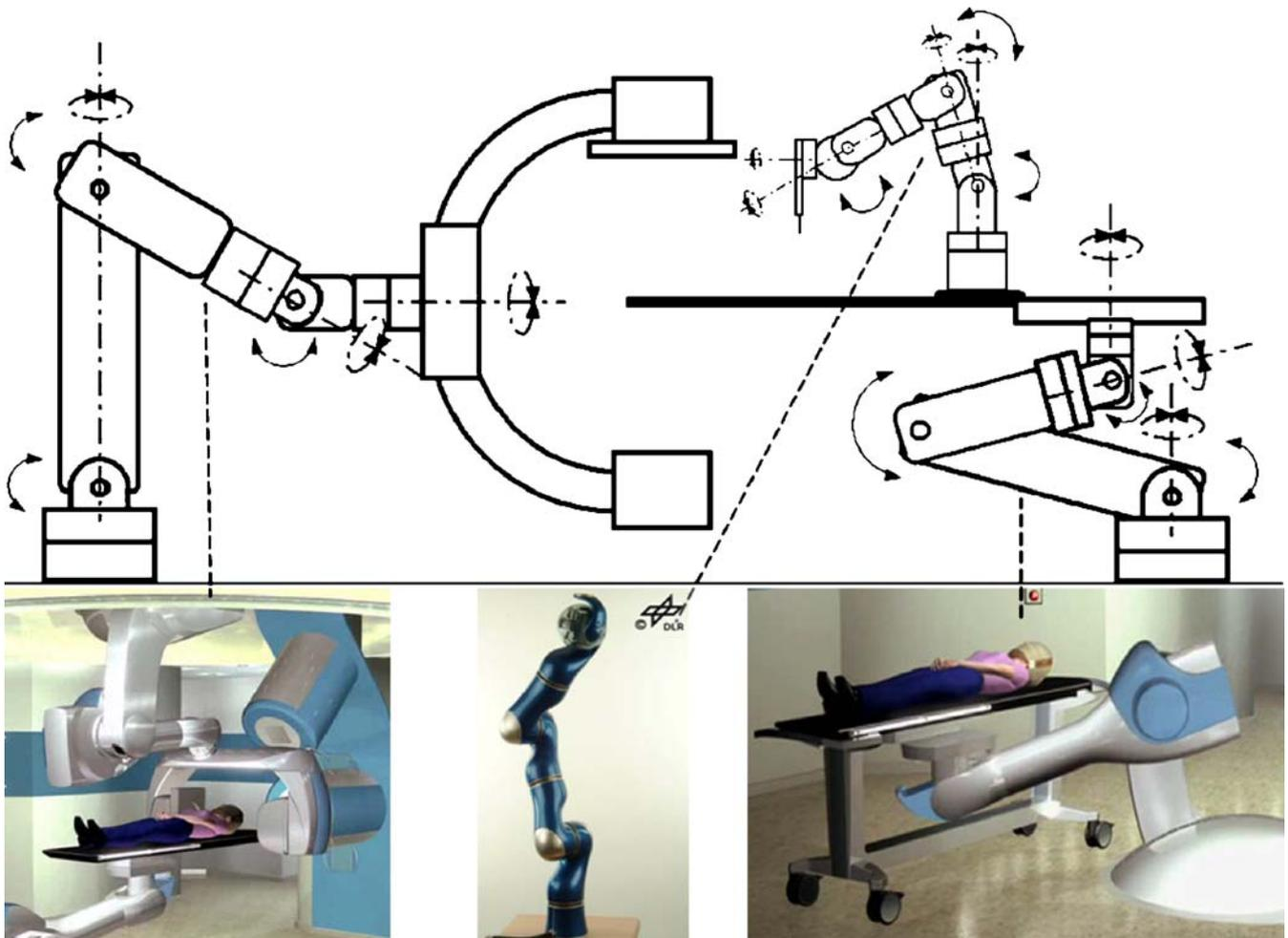
**Fig. 8** Potential future developments in FD-CT: robots will allow for faster, more precise and more flexible data acquisition and therapy (see text). (Renderings of the two large robots are a courtesy of Siemens Medical Systems Particle Therapy Division)
