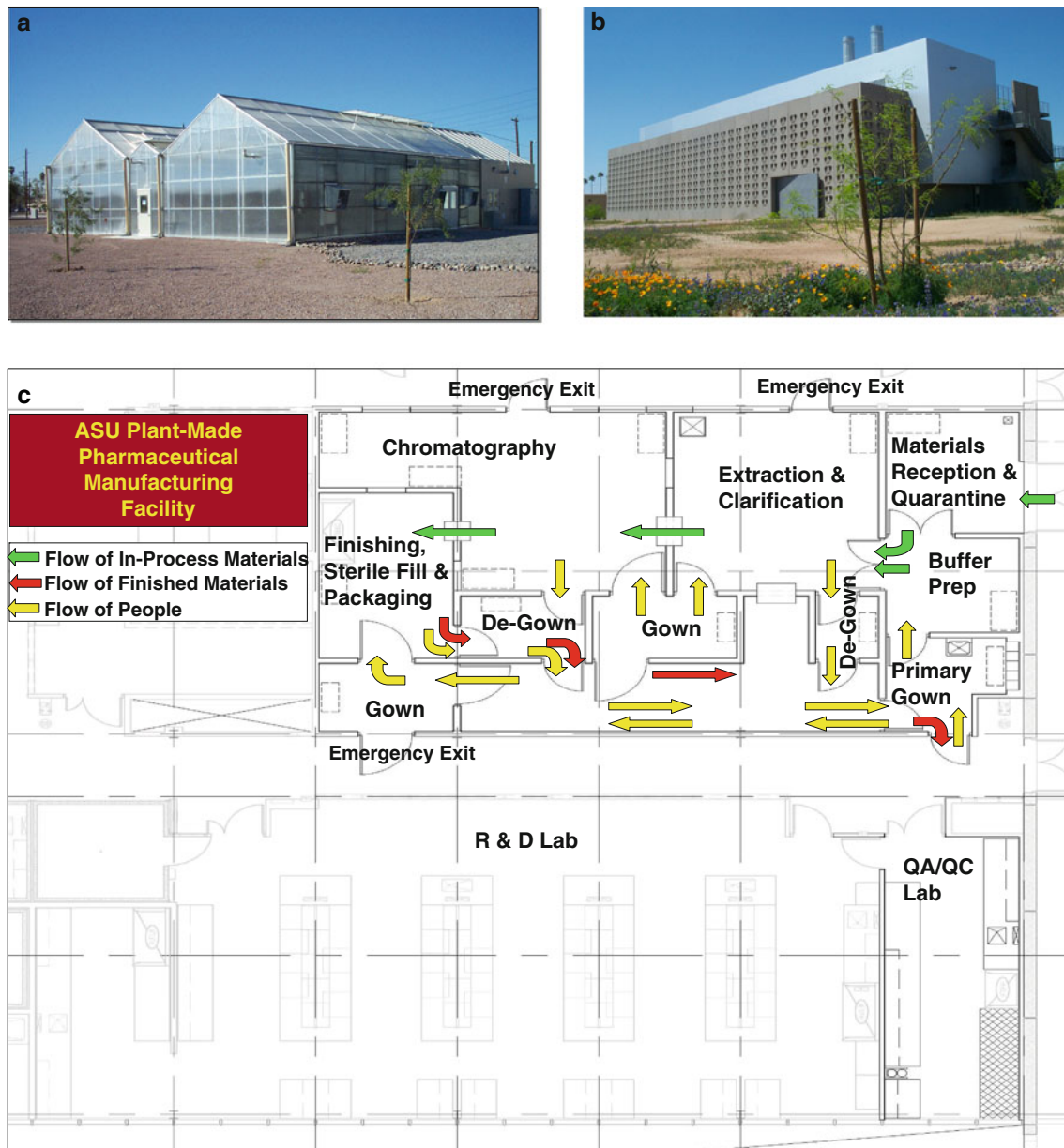
Fig. 1 Facilities for cGMP production of NVCP VLP vaccine and other plant-made pharmaceuticals. a The 3,600 ft 2 BSL-2 greenhouse facility for plant biomass generation and NVCP expression. b The plant biopharmaceutical center that houses the central bioprocessing
