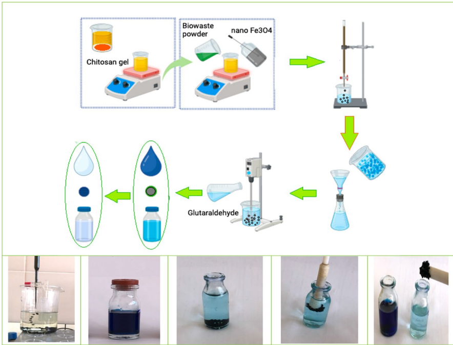
Fig. 2 Schematic diagram of preparation of m-WCH and m-OCH and adsorption of MB
