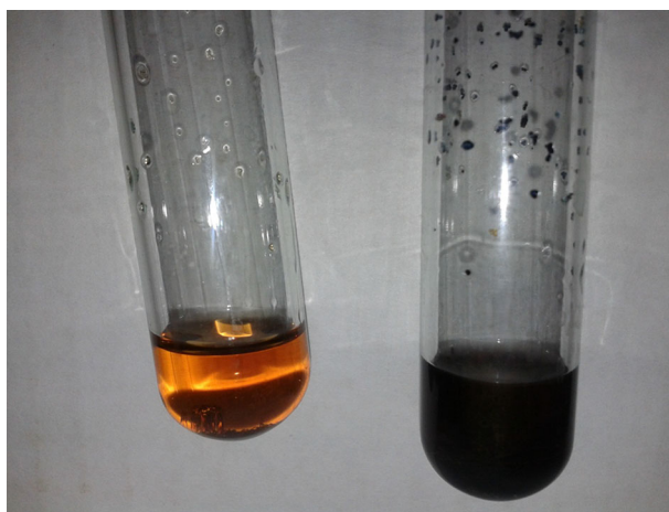
Fig. 4 The Kaiser's procedure performed on the resin 1S. The test tube on the left contains test solution, the one on the right is the solution with the sample added
