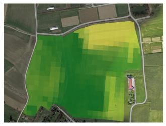
**Fig. 3** Prescription map created with a software tool. The field is split into grid squares which each require a different level of product applied to them
