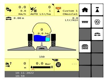
**Fig. 2** Image of a universal terminal (UT) display. The large area on the left is a square-shaped data mask where information is displayed. The right side is reserved for soft-key icons which are used for navigation, and control of the machine. For each soft-key, a mechanical push button is associated—today mechanical buttons are commonly replaced by touch-screen capability
