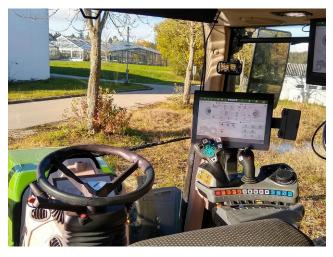
Fig. 1 The inside of a modern tractor cabin. The main terminal can be seen behind the joystick
