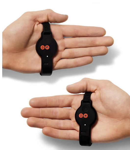
Figure 5. A force sensor band. (Credit: eo SwimBETTER.)
