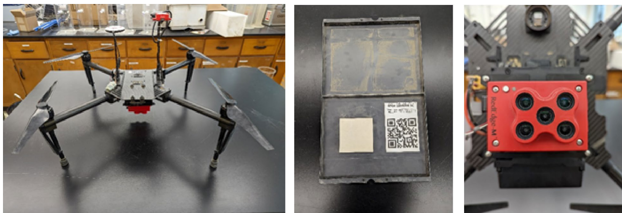
Fig. 2 Left to Right: DJI Matrice 100, Micasense Reflectance Calibration Panel, and Micasense RedEdge Multispectral Camera
