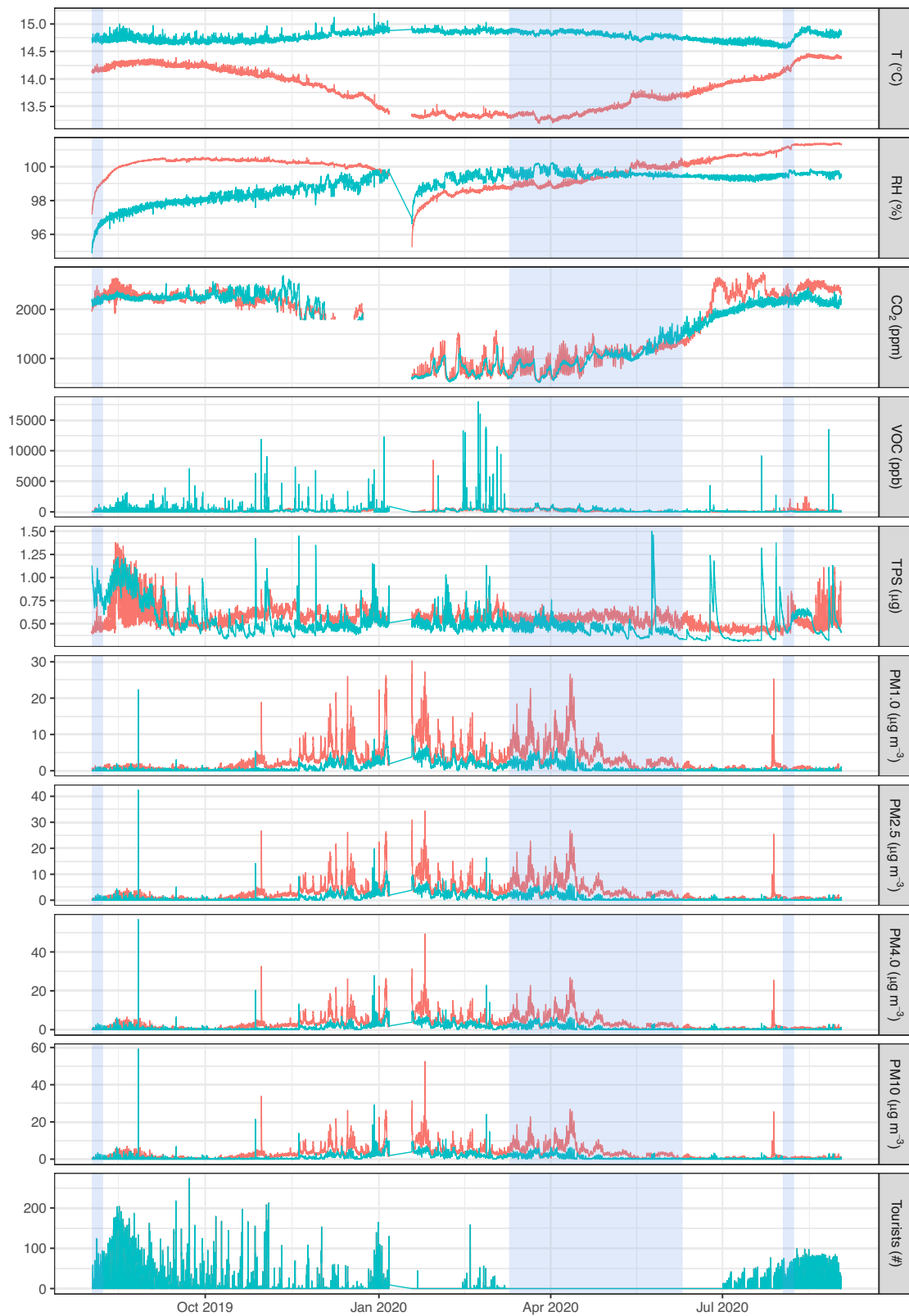
Fig. 2 Time series of all the parameters monitored (temperature: T, relative humidity: RH, CO 2 , VOC, typical particulate size: TPS, PM1.0, PM2.5, PM4.0, PM10) in the tourist (green) and fossil (red) trails, as well as the number of tourists in the cave. Shaded areas
