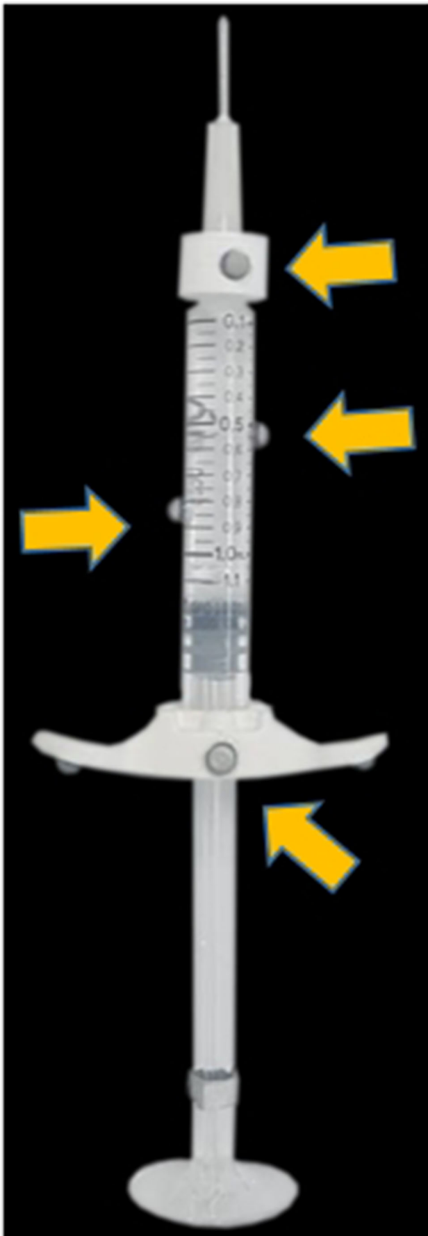
◀ Fig. 6 The model of the syringe is shown. An actual hyaluronic acid filler syringe was used and passive markers (yellow arrows) were attached to it. The filler product is from Sthepharm Co., Ltd. (Seoul, Republic of Korea)
