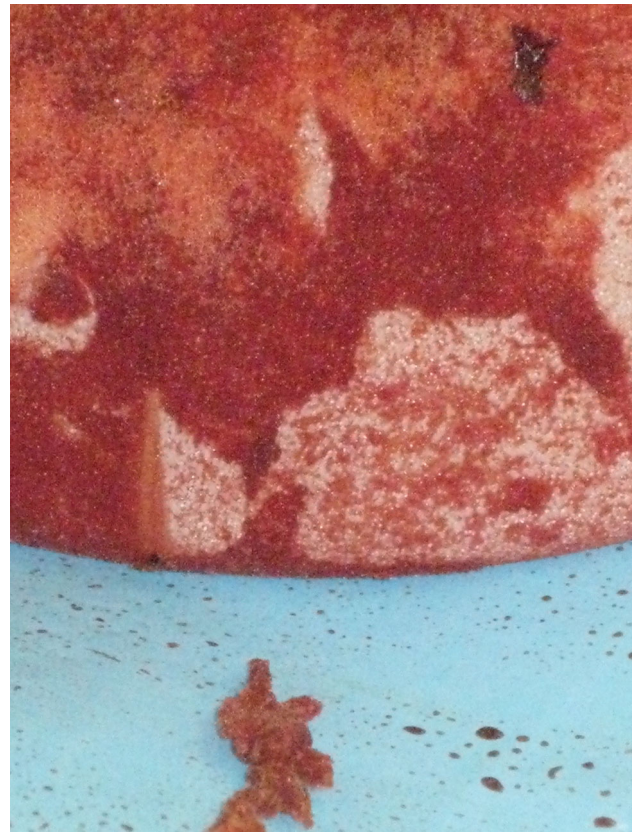
Fig. 1 Early delamination of polyurethane foam from a Silimed implant
