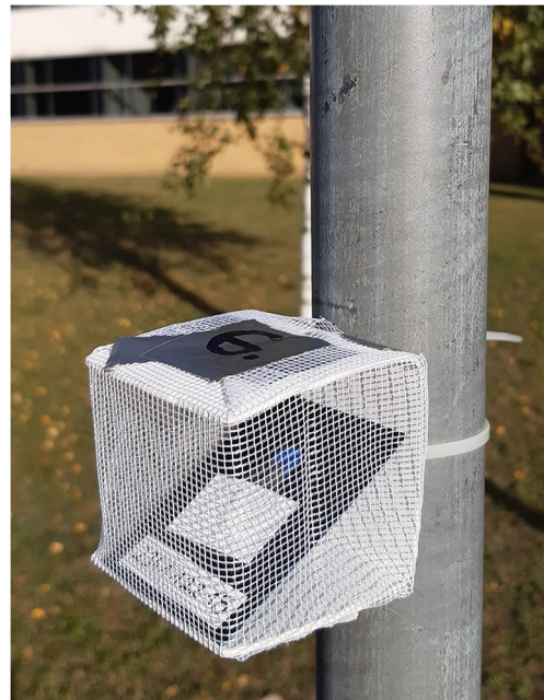
Fig. 1 Example of a feather sample and box used in the exposure experiment
