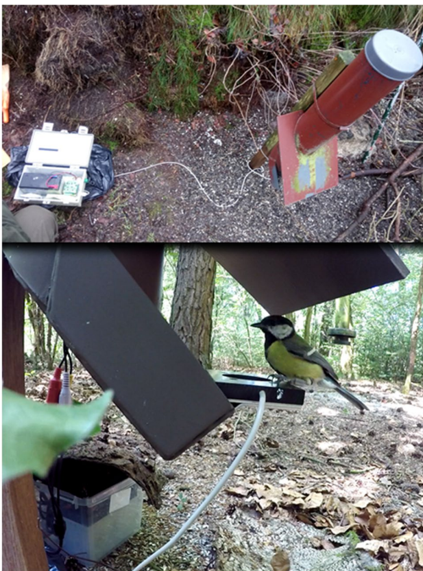
Fig. 2 One of the feeders distributed in Westerheide study area during winter 2018–2019. Above: feeder tube attached to a pole, connected to the printed circuit board, RFID reader, and 12 V battery. Below: great tit at the feeder access, perched on the reader antenna
