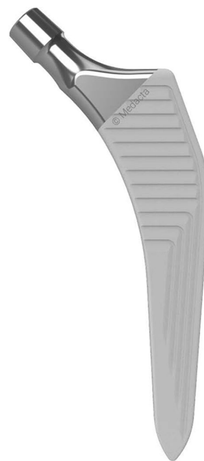
Fig. 1 AMIStem-H (referred to as Original stem) (Medacta, Switzerland) first undergoes a sandblasting process to roughen the entire surface of the stem to 2.5–6 \mu\text{m} ; then, it is fully coated with an 80 \mu\text{m} layer of HA
