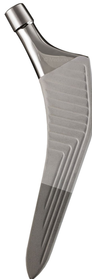
Fig. 2 AMIStem ProxCoat (referred to as ProxCoat stem) (Medacta, Switzerland) first undergoes a sandblasting process to roughen the entire surface of the stem to 2.5–6 \mu\text{m} ; then, the proximal two-thirds of the stem are coated with a 300 \mu\text{m} layer of MectaGrip (unalloyed titanium with a pore size of 100–350 \mu\text{m} ) through Air Plasma Spray (APS) technology, and finally, the proximal two-thirds of the stem are coated with an 80 \mu\text{m} layer of HA
