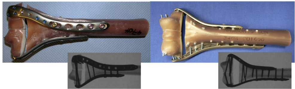
Fig. 1 Examples for the 90° ( left ) and 180° ( right ) configuration and fracture design
