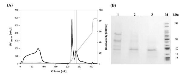
**Fig. 1** Anion exchange (HiTrap QFF 5 mL) chromatogram (**A**) of concentrated BMMY supernatant after ~96 h of induction with methanol. Pooled fractions with *Tc*-LysN activity are enclosed within two straight lines. Sodium dodecyl sulfate–polyacrylamide gel electrophoresis (**B**) of the *Tc*-LysN purified from culture supernatant via AEX. Lane M contains the marker proteins (broad range
