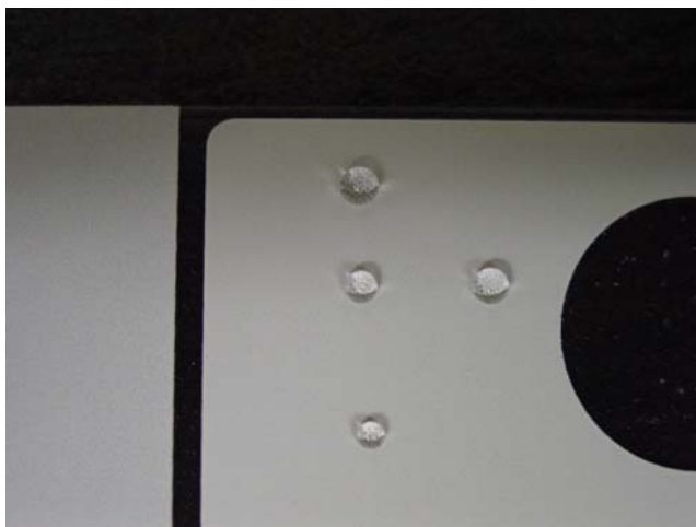
Fig. 1 Image of four droplets deposited onto a teflon-coated surface
