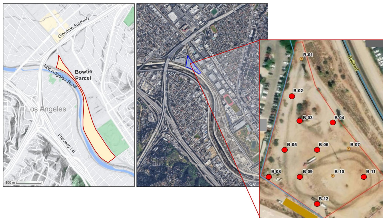
Fig. 1 Study site and sampling design. Aerial view of the sampling location, known as the “Bowtie” property within Taylor Yard—a former rail yard in Los Angeles, CA, that is owned and managed by California State Parks. Soil samples were taken from below ground (at 0.1524 m, 1.524 m, 3.048 m, 4.572 m, and 6.096 m) at 12 ordinary
