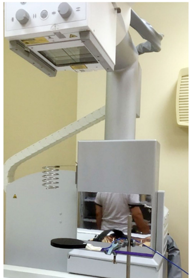
Fig. 2 A photograph shows a Siemens dRF radiographic unit and the 75-cm 3 pancake chamber
