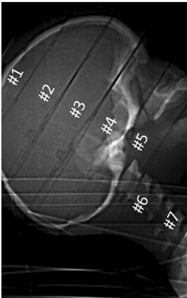
Fig. 2 Phantom sections in a lateral topogram image. Due to the inclination of the head, different sections are exposed in the frontal and occipital regions
