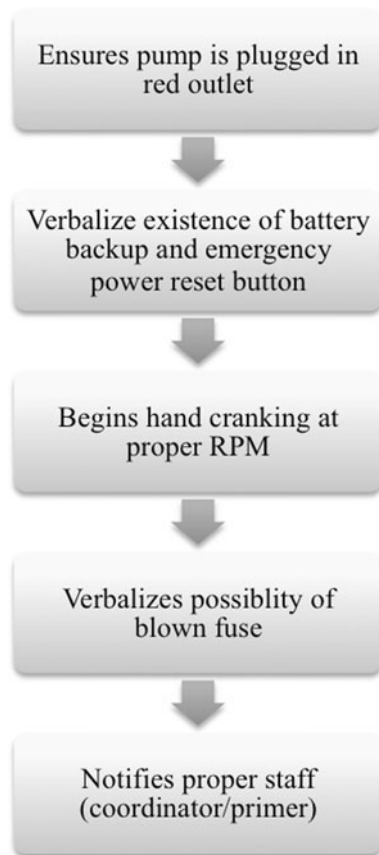
Fig. 4 Flow chart of the critical performance criteria in a power failure emergency scenario
