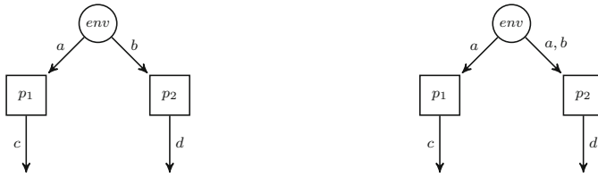
(a) An architecture of two processes that specify process p_1 to produce c from a and p_2 to produce d from b . (b) The same architecture as on the left, where the inputs of process p_2 are changed to a and b .
