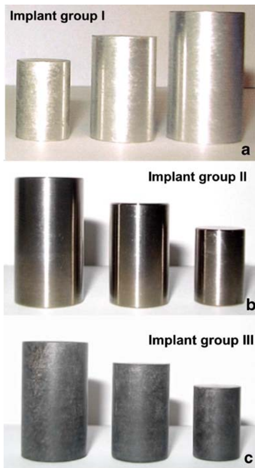
Fig. 1 a–c Cylindrical EST implants. a Magnesium (implant group I). b Titanium (implant group II). c CFRP (implant group III)
