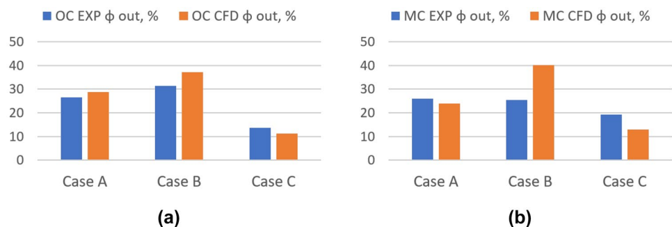
Fig. 12 Outlet relative humidities: (a)—OC; (b)—MC; OC—original construction; MC—modified construction; EXP—experimental value; CFD—numerically obtained value
