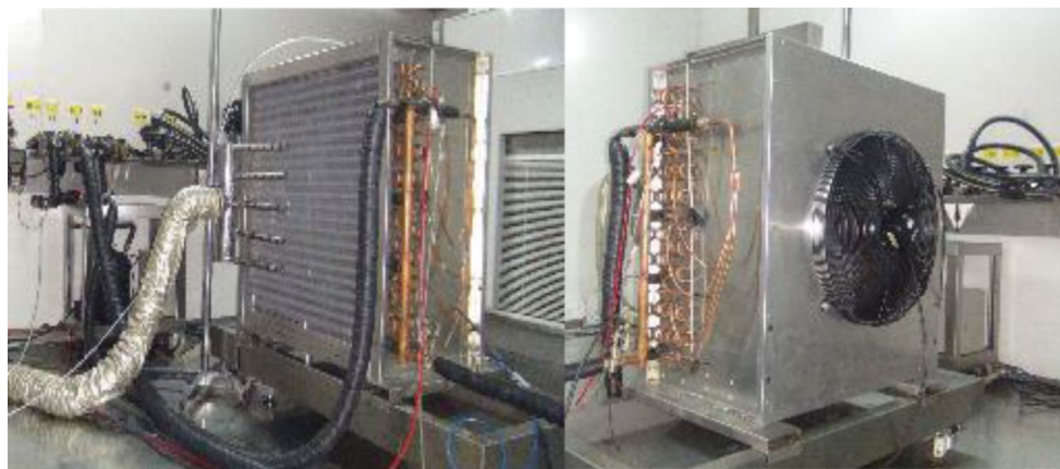
Fig. 1 The general view of the unit cooler inside the calorimetric room at Friterm R&D laboratory
