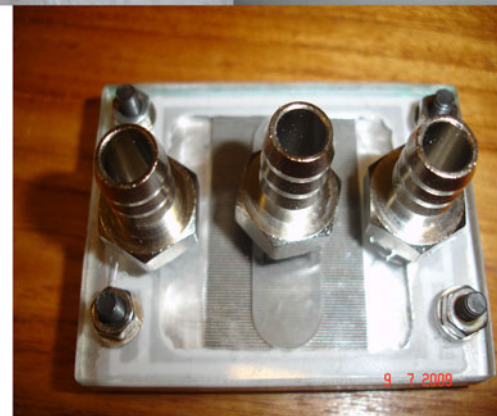
Fig. 2 Photograph of the micro fin heat sink components
