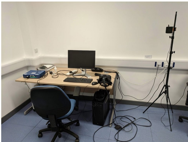
Fig. 3 Laboratory set-up with HTC Vive headset (right-hand side of desk) and front base station (far right of image); the rear base station (not pictured) was placed on the left behind the desk chair facing both the desk and front base station
