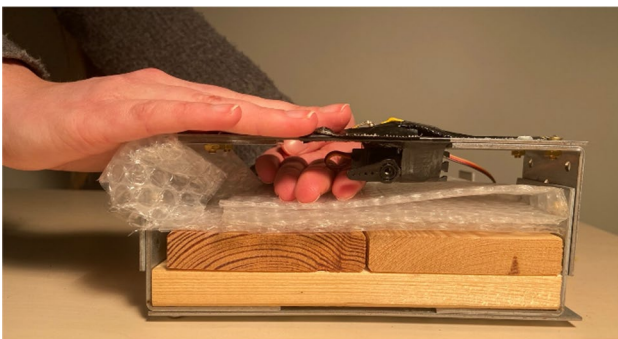
Fig. 1 Experimental setup. The left hand was placed underneath the motor which was attached to a metal arch. Once the auditory go signal occurred, participants were instructed to press the force sensor with the right index finger which led to the left index finger being touched by a lever controlled by the motor
