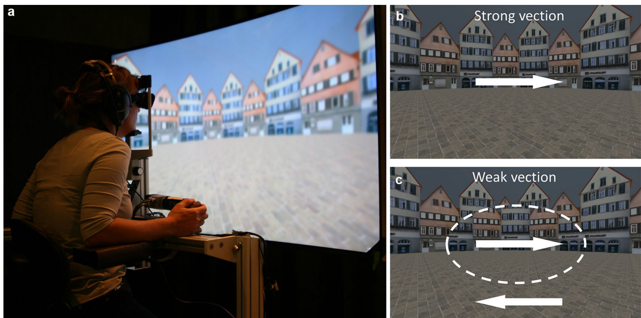
Fig. 1 a Experimental setup; b strong-vection condition, with scene moving coherently; c weak-vection condition with ellipse-shaped central part (dashed line) moving opposite to the periphery. Arrows indicate direction of scene motion
