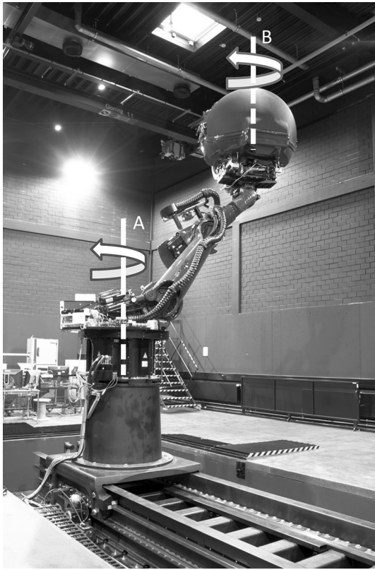
Fig. 3 CyberMotion simulator in the configuration for the circular trajectories. During the trial, the cabin was rotated using the main centrifuge axis (a); Only after the trial, the cabin was reoriented using the cabin yaw axis (b)
