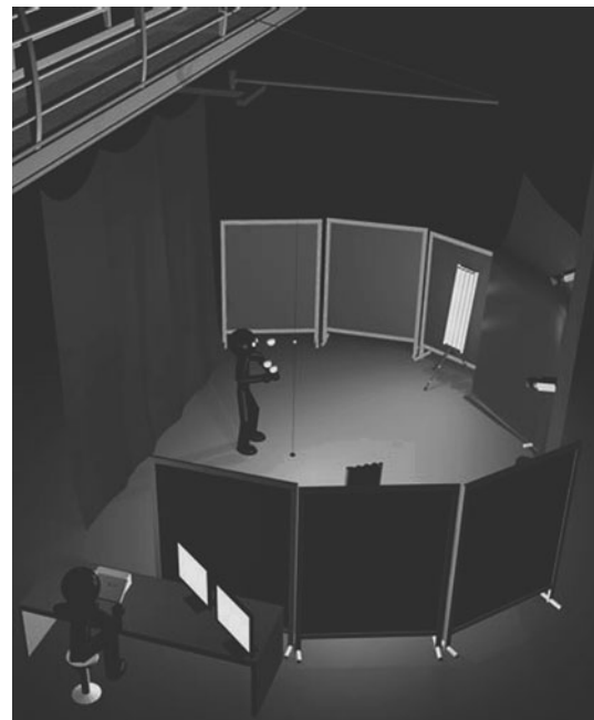
Fig. 2 Cartoon of the experimental setup, showing the lever, fishing line, and bead used to present the fixation point in front of the participant
