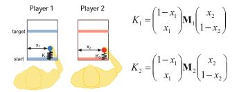
Fig. 1 Experimental setup. Player 1 and Player 2 each control a cursor from a start bar to a target bar. The movement can be chosen anywhere along the x-axes. However, the forces that resist the players' forward movement are given by spring constants whose stiffness depend both on the x-position of Player 1 and on the x-position of Player 2
