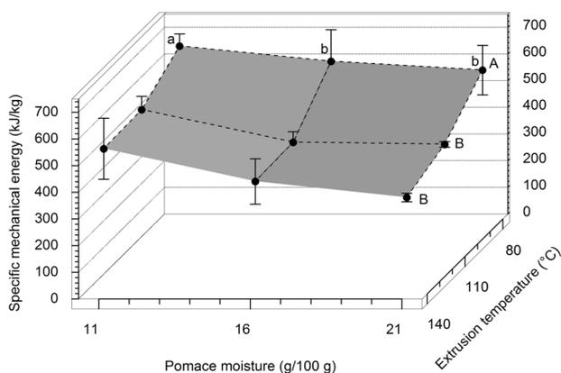
**Fig. 1** Specific mechanical energy during extrusion of seedless blackcurrant pomace at different temperature and varying moisture content. Lowercase letters indicate significant differences ( $p < 0.05$ ) caused by pomace moisture; uppercase letters indicate significant differences caused by extrusion temperature ( $p < 0.05$ ); the interaction of the parameters moisture and temperature was insignificant
