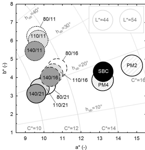
**Fig. 2** Colour coordinates of seedless blackcurrant pomace (SBC) as affected by extrusion conditions (encoded with temperature [°C]/pomace moisture [g/100 g]) or planetary ball milling for 2 h (PM2) or 4 h (PM4). Lightness  $L^*$  is proportional to circle area as indicated
