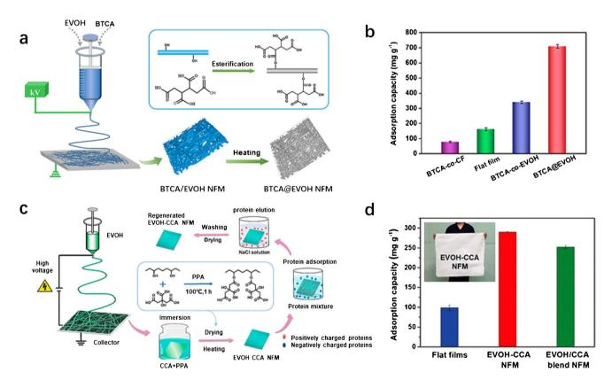
**Fig. 5** The preparation and functionalization process of BTCA, CCA grafting agent EVOH nanofibrous membranes, and adsorption capacity. **a** Prepared BTCA@EVOH NFM and modification principle. **b** BTCA@EVOH NFM comparison of adsorption capacities with flat
