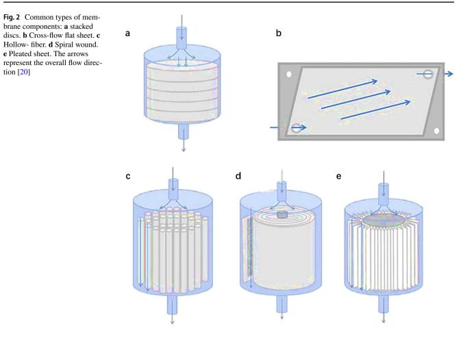
Membrane adsorbers usually adopt hollow fiber, flat plate (usually disc shape), radial flow, spiral winding, cylindrical plug, and other membrane forms (Fig. 2) [20, 21]. Most of the membrane adsorbents are stacked, among which hollow fiber and stacked disc membrane adsorbents have been used in commercial applications. The radial flow and cross-flow membrane modules are easier to be applied in large-scale industrial production because they are difficult to produce membrane fouling.
