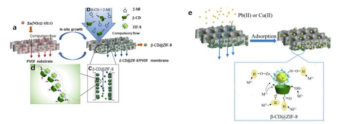
Fig. 10 a assembly of Zn(II) on the PVDF: fabrication of the  $\beta$ -CD@ZIF-8/PVDF. b Assembly of ZIF-8 and formation of  $\beta$ -CD. c Structure of the membrane. d Sketch map of  $\beta$ -CD@ZIF-8 binding. e Adsorption mechanism of the Pb<sup>2+</sup> and Cu.<sup>2+</sup> [132]
