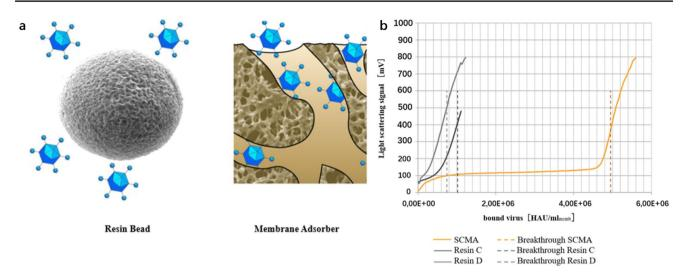
Fig. 3 a Adsorption model of the virus on traditional resin surface and SCMA membrane. b Comparative evaluation of SCMA membrane and commercially available sulfated cellulose resins [62]
