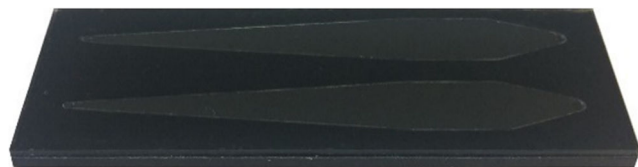
Fig. 2 Ready-to-use microfluidic chip (flow direction from left to right)
